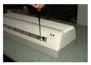
③ Detach the attachment tabs (2) at the top of the grille by lifting the grille.
